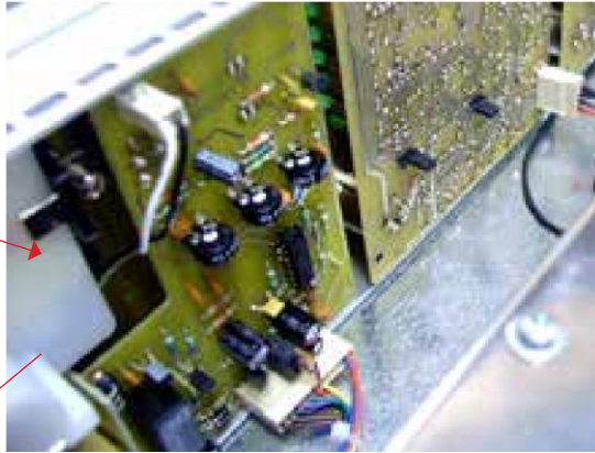
Audio card with digital filter and limiter
